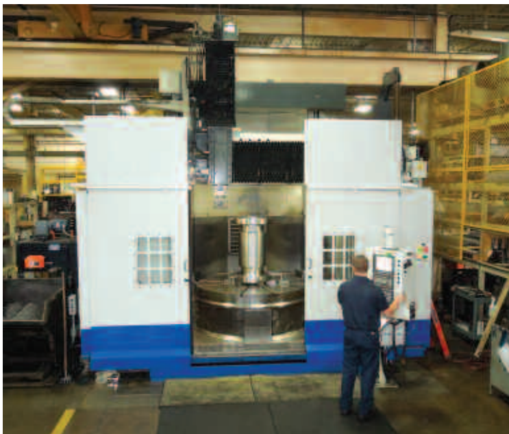
Vertical turning capacity from 30" to 84" diameter.
